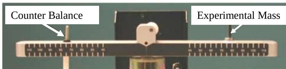
Figure 2: Rotating arm of the Centripetal Force Apparatus. The Experimental Mass is held in place when masses are secured to the top. The Counter Balance can slide freely even when masses are secured in place. (Image from PASCO ME-8088 Instructions).
